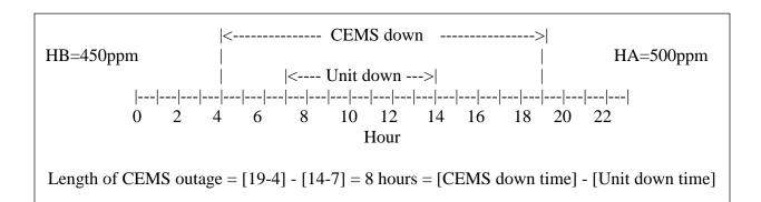
Assume that the PMA of the  $SO_2$  monitor is  $\geq 95\%$ . As illustrated above, the missing data period is 8 hours, when the unit downtime is excluded.
