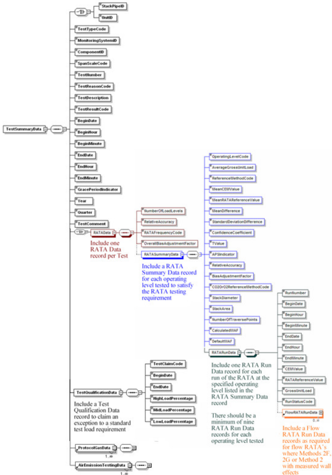
Figure 16a RATA Test XML Structure
