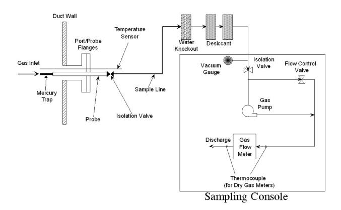
Figure 30B-1. Typical Sorbent Trap Sampling System
